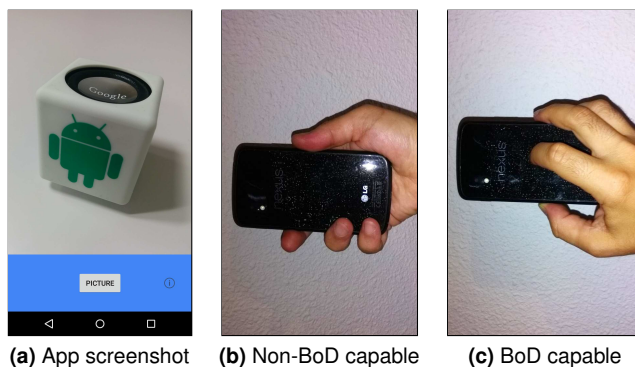
Figure 2: The \beta Tap camera app (a) allows for a more comfortable holding; cf. (b) vs. (c).
